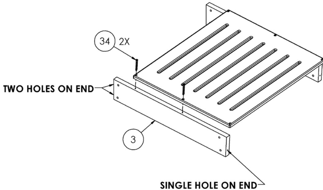
3. Attach part (4) to assembly with screws (34).
