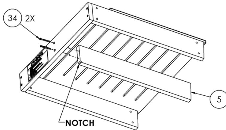
5. Attach part (6) to assembly with screws (34).
