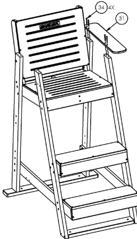
24. Attach arm rest (32) using screws (34).
