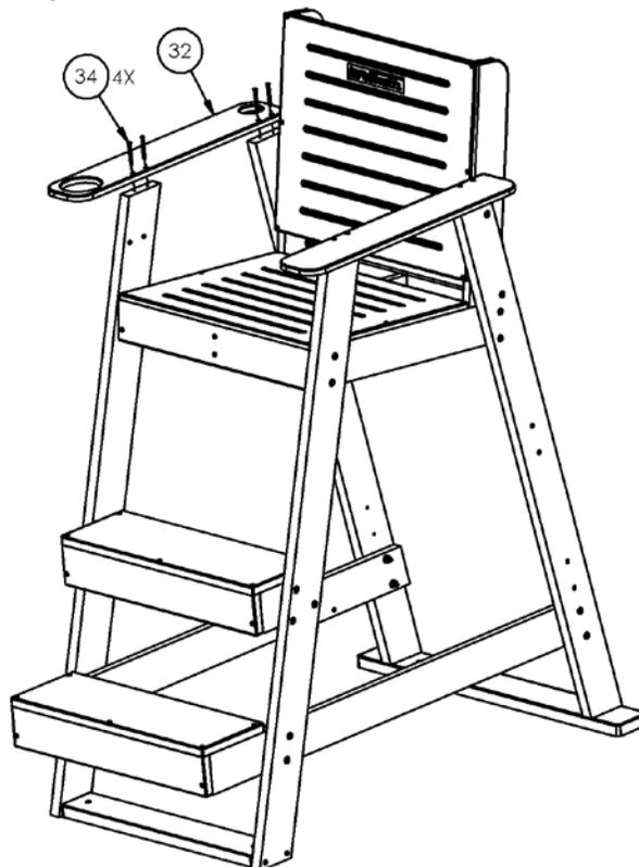
25. Attach braces (24) using screws (34).
