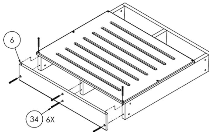
6. Seat Bottom Assembly should look like the pictures below when finished. Next make Seat Back Assembly.
