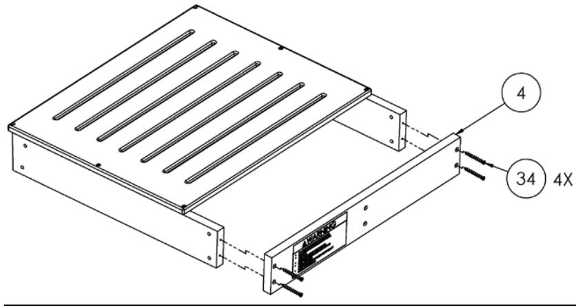
4. Attach part (5) with notch in direction shown to assembly using screws (34).
