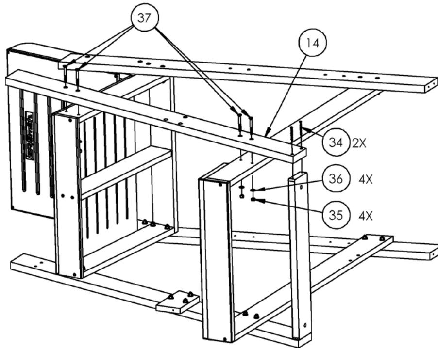
20. Now install the other step side (23) using nuts (35), washers (36), and screws (37).
