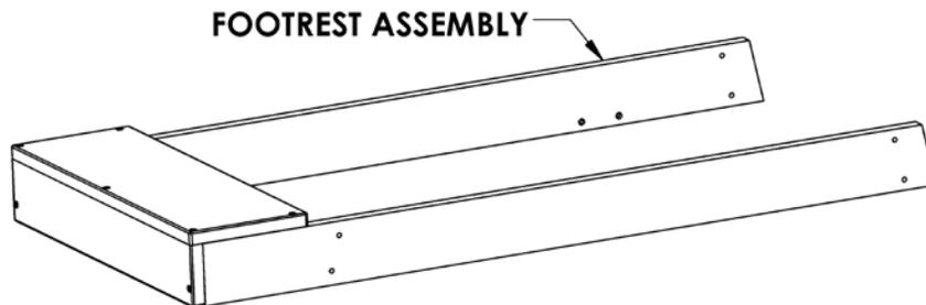
14. Attach Seat Back Assembly, Seat Bottom Assembly, and Footrest Assembly to leg (15) as shown using nuts (35), washers (36), and screws (37).
