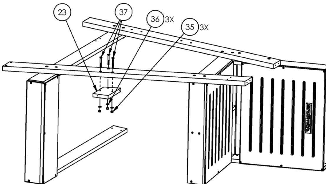
17. Now flip the chair over and attach leg (16) to assembly using nuts (35), washers (36), and screws (37).
