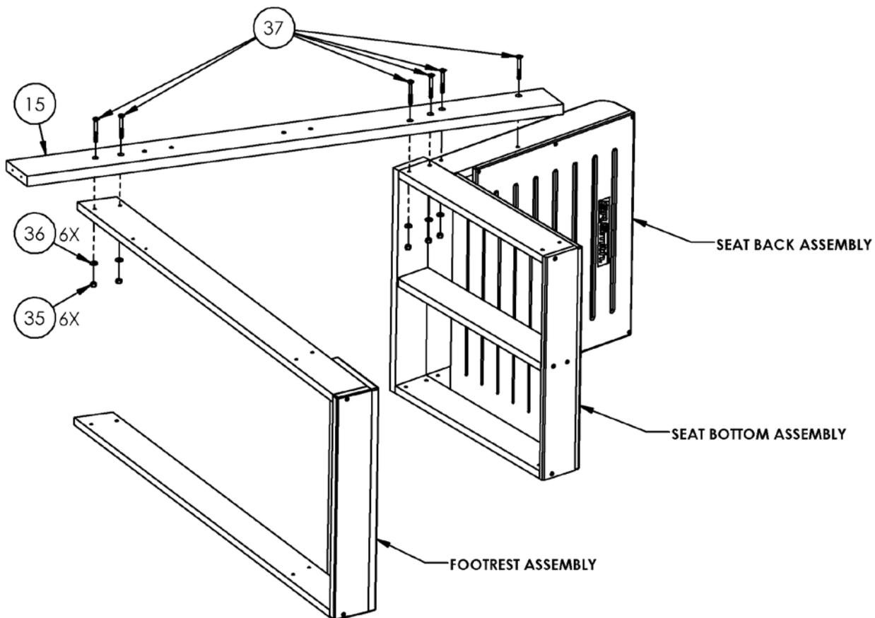
15. Next, attach leg (13) to assembly using nuts (35), washers (36), and screws (37).
