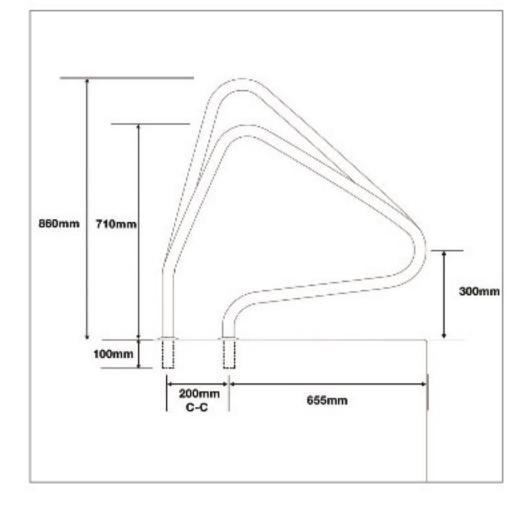
The AQUEAS AQ-GR05 uneven rails are well suited to commercial applications when niche steps are used with pool grates. The uneven rails catering for people of different heights and making it difficult to slide down them making it safer. This can be used for residential applications as well.
