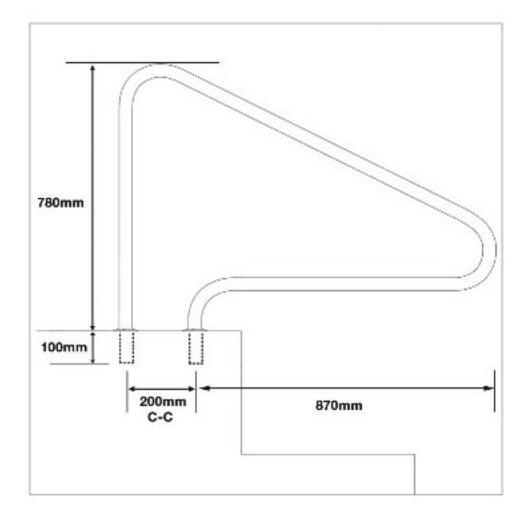
The AQUEAS AQ-GR02 extended rails are well suited to residential applications that have steps. This can be used for commercial applications as well.
