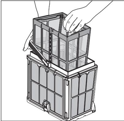
**6.2.1** Hold down the handle to remove the inner net basket.
