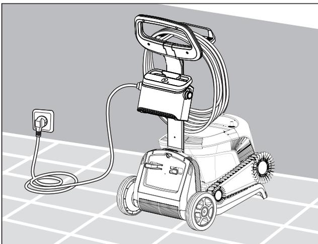
**5.3.1** Hang the power supply on the Caddy adaptor for power supply and plug it into the wall outlet.
