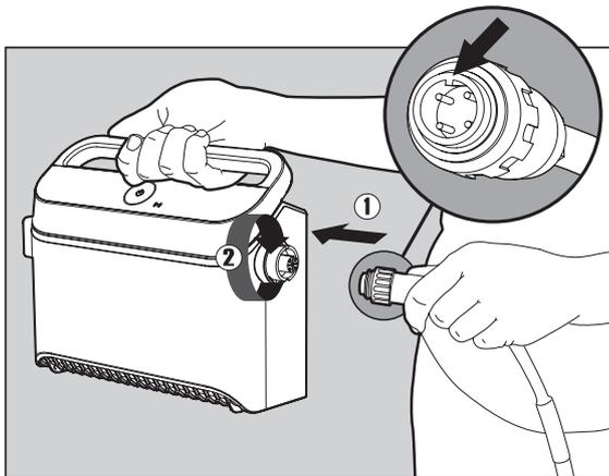
**5.1.3** Attach the blue cable to the power supply: Insert the cable with the notch on the connector (1), lined up with the groove in the socket on the power supply, and turn clockwise (2).
