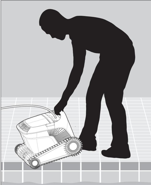
**5.2.1** Place the robotic pool cleaner in the pool. Release it and let it sink to the floor of the pool. Make sure that the blue cable is free of any obstacles.
