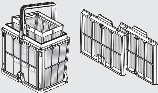
\* The filter panels are assembled on the filter basket.
