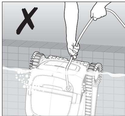
Use the cable to pull the robotic pool cleaner to the side of the pool. Use the handle to remove the robot from the pool.
