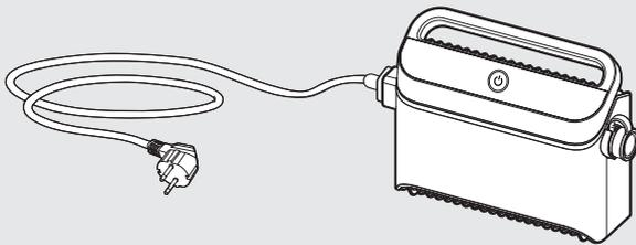
The power supply unit is designed to be resistant to rain but it is not sealed from moisture. Like any other electrical device, we recommend covering it during wet seasons.
