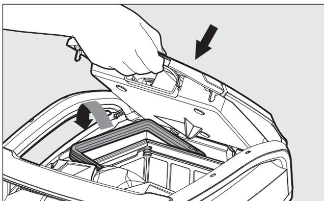
**6.2.6** Reposition the inner net basket, check that each filter was placed well, and insert the clean filter basket. Close the filter cover.
